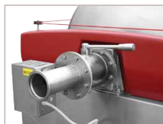
overfilling signalisation, axial filling valve
