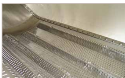
connected draining channels, electropolished
